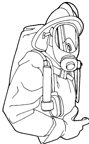
A mask and a respirator for a firefighter protect against debris, gas, heat and smoke.
